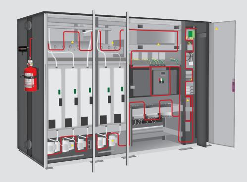
When installing a direct low pressure system on a capacitor cabinet or converter cabinet, route the flexible detection tubing around all possible ignition sources.
